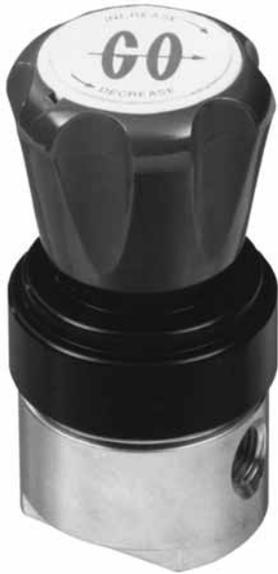
The PR-2 Series are compact, brass body regulators designed for maximum flexibility in many classes of instrumentation service. Specifically designed for gas applications, this regulator is capable of accepting high pressures directly from cylinders and other high pressure, non-corrosive systems. It is ideally suited for carrier gas pressure regulation, and is economical enough to use in low pressure air systems, such as instrument cabinet air purge service.
